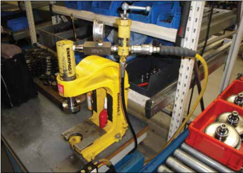
▲ RC-308 cylinder mounted in A-330 Arbor Press powered by a PATG-Turbo Air pump for controlled pressing of bearings for sprockets of weaving machines. The V-152 Pressure Relief Valve controls the pressing force.
