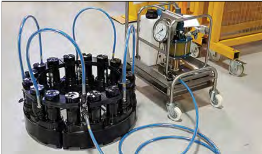
▲ Multi-Stud Tensioning Set-Up.
