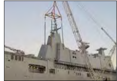
Synchronous hoisting and load positioning
