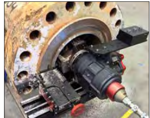
▼ MM860I machine to ensure flange joint integrity.
