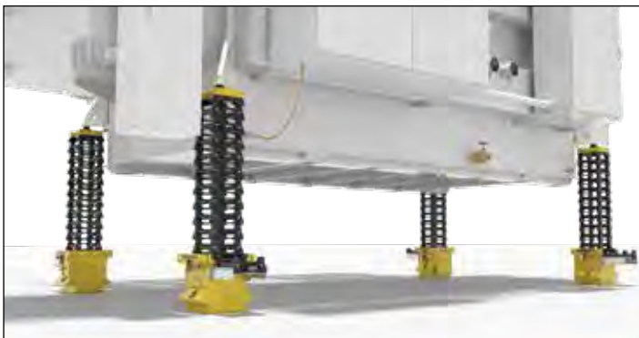
▼ Typical set-up with 4 Self-Locking Cube Jack and cribbing blocks to lift a transformer (hydraulic power pack and hoses not shown).
