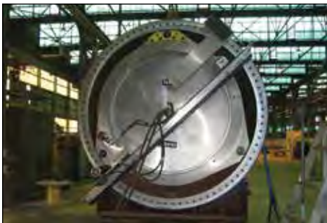
▼ Wind tower machining with WP4600.
