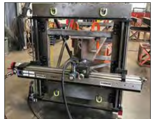
I-Beam end face milling with a GMRF1000. ▶
