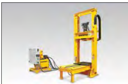
◀ 100-Ton Press for Assembly of Spring-Loaded Cylinders
