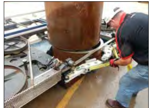
▲ Pipe cutting with BS portable band saw.
