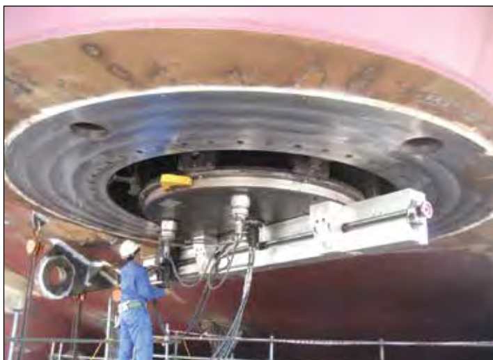
▼ Milling a ship thruster flange.
